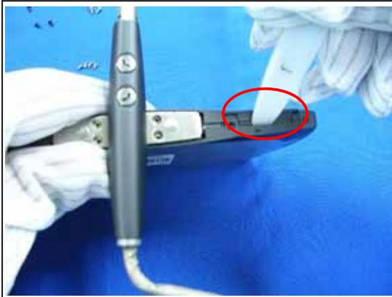
Insert plastic stick into the right side gap between LCD housing and bezel.
