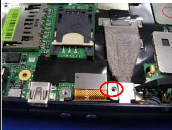
Assemble LCD coaxial cable cover and fasten one screw to fix it.
