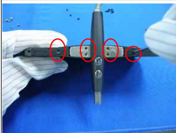
Fasten 6 screws on LCD module.
