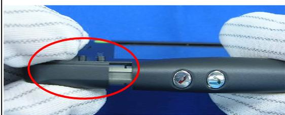
Disassemble cover hinge-Left.
