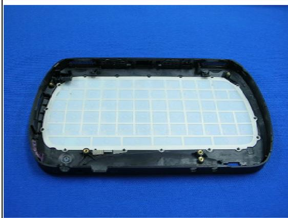
Assemble keypad into bezel.
