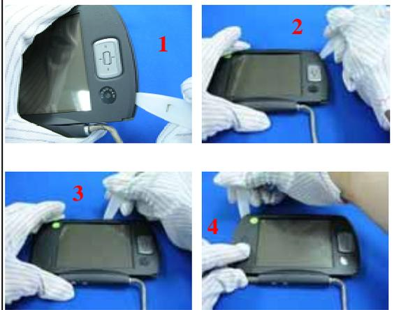
Follow the sequence to release 8 hooks between LCD bezel and housing, then remove LCD housing.
