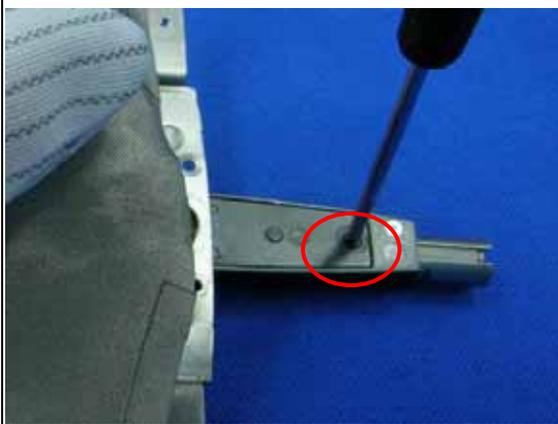
Fasten one screw to fix LCD cable with cover hinge.
