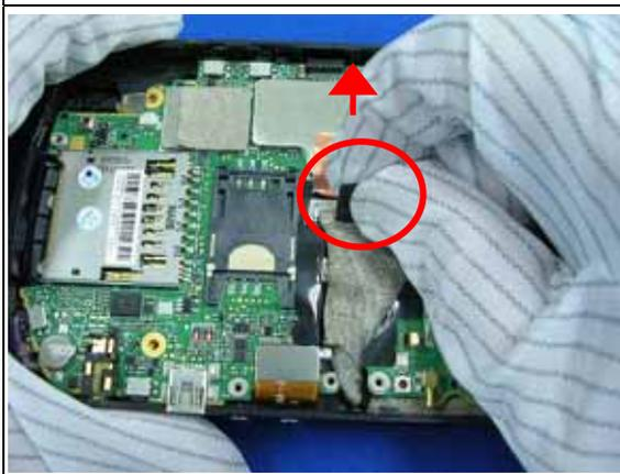
Pull out LCD coaxial cable (Display).
