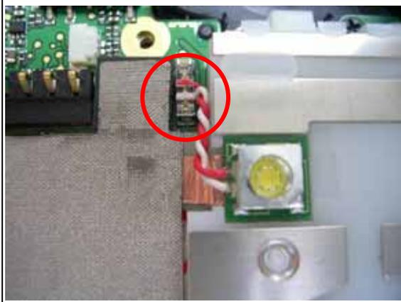
Release the flashlight connector, then remove the flashlight.
