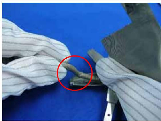
Release the cable from cover hinge.
