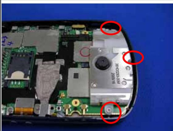
Assemble the antenna and fasten 3 screws to fix it.
