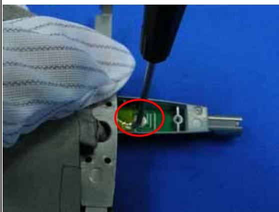
Fasten one screw to fix LED board.
