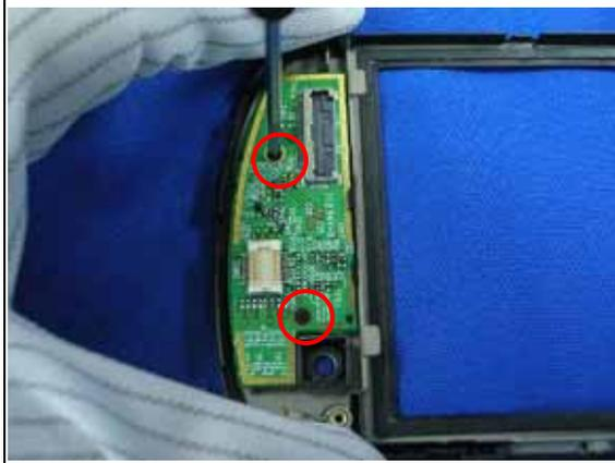
Assemble upper cover board, and fasten 2 screws to fix it.
