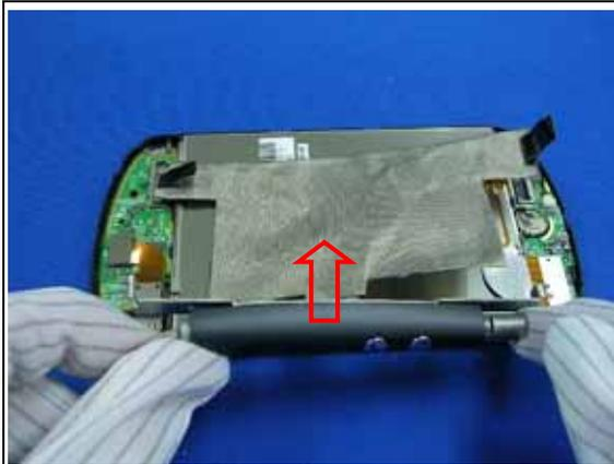
Remove LCD coaxial cable module.
