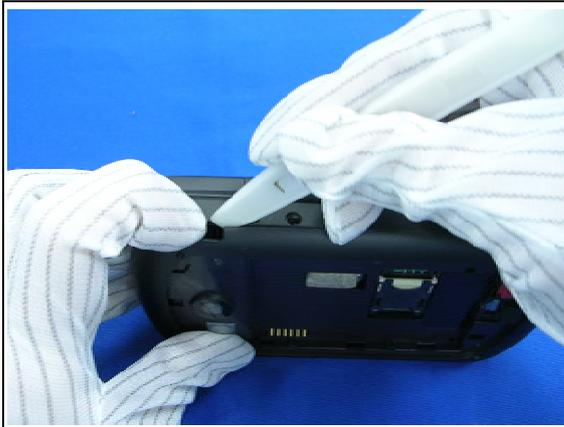
1. Insert the plastic stick in the gap between the bezel and housing deep inside.
