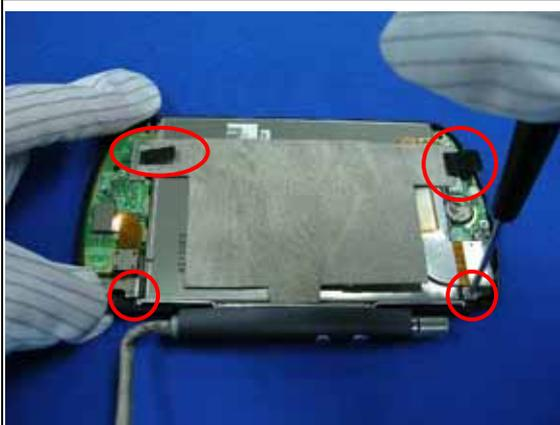
Connect cable with upper cover board and lower cover board.
