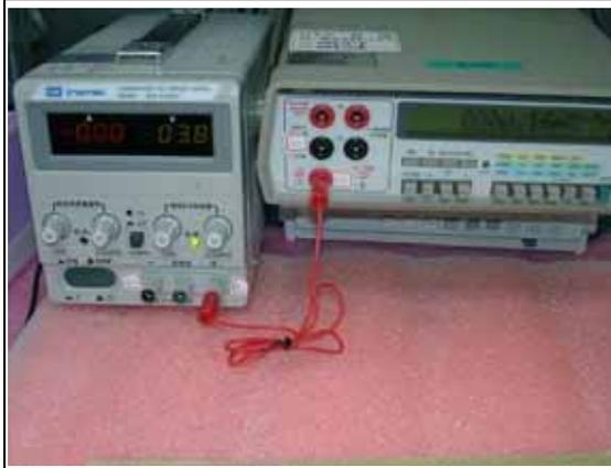
3. Connect cable (D) to positive polarity of power supply (A) and current meter (B)
