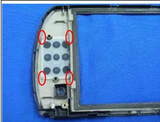
Assemble navigation button to LCD bezel.
