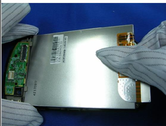
Assemble LCD into bezel.
