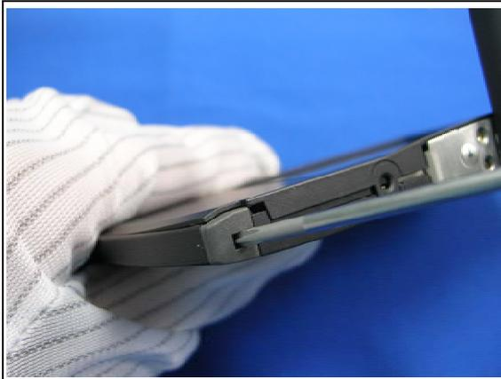
Insert screw driver into the hole and press to release the hook.
