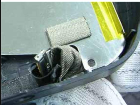
Assemble LCD coaxial cable through into keypad bezel.
